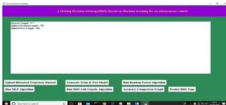
FIG 4 In above screen dataset contains 977 total trajectory records and application using 781 (80% of dataset) records for training and 196 (20% of dataset) for testing. Now both training
